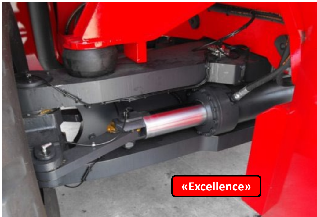
Sandwich (I-beam) style steer axle
